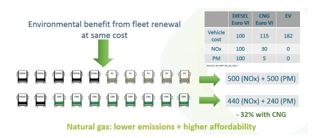
Comparison of Diesel fleet renewal with Electric vehicles and Gas-fuelled vehicles at the same cost.
